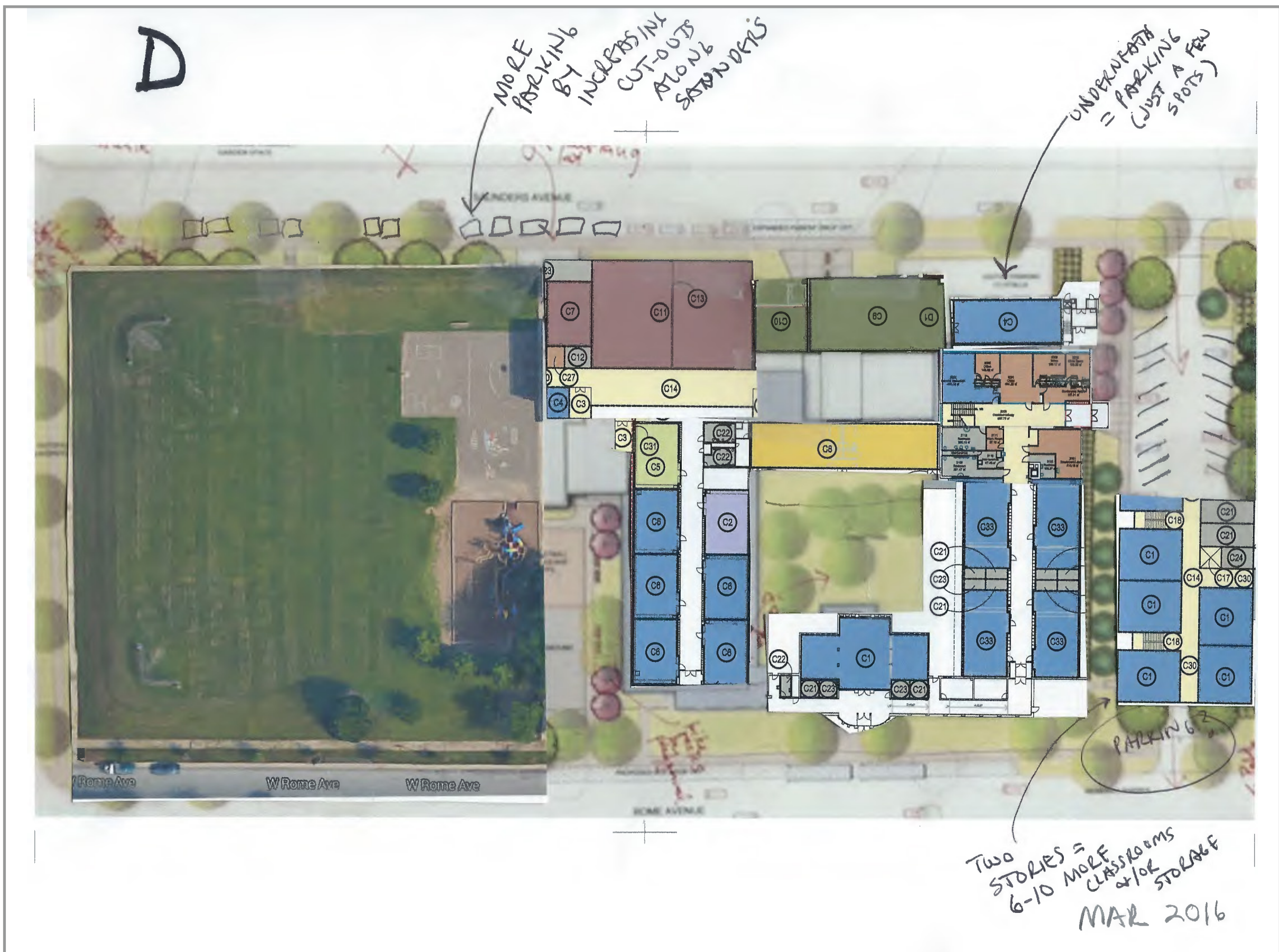
Sketch D: This has more detail and shows how the back part of the proposed parking can accommodate two stories of classrooms. The Saunders side of the school could have parking underneath an expanded administrative office space or the enlarged cafeteria. The existing gym can be expanded toward Saunders and toward Davern without taking away from the open field. Again, the translucent roof over the corridor will add natural light.
