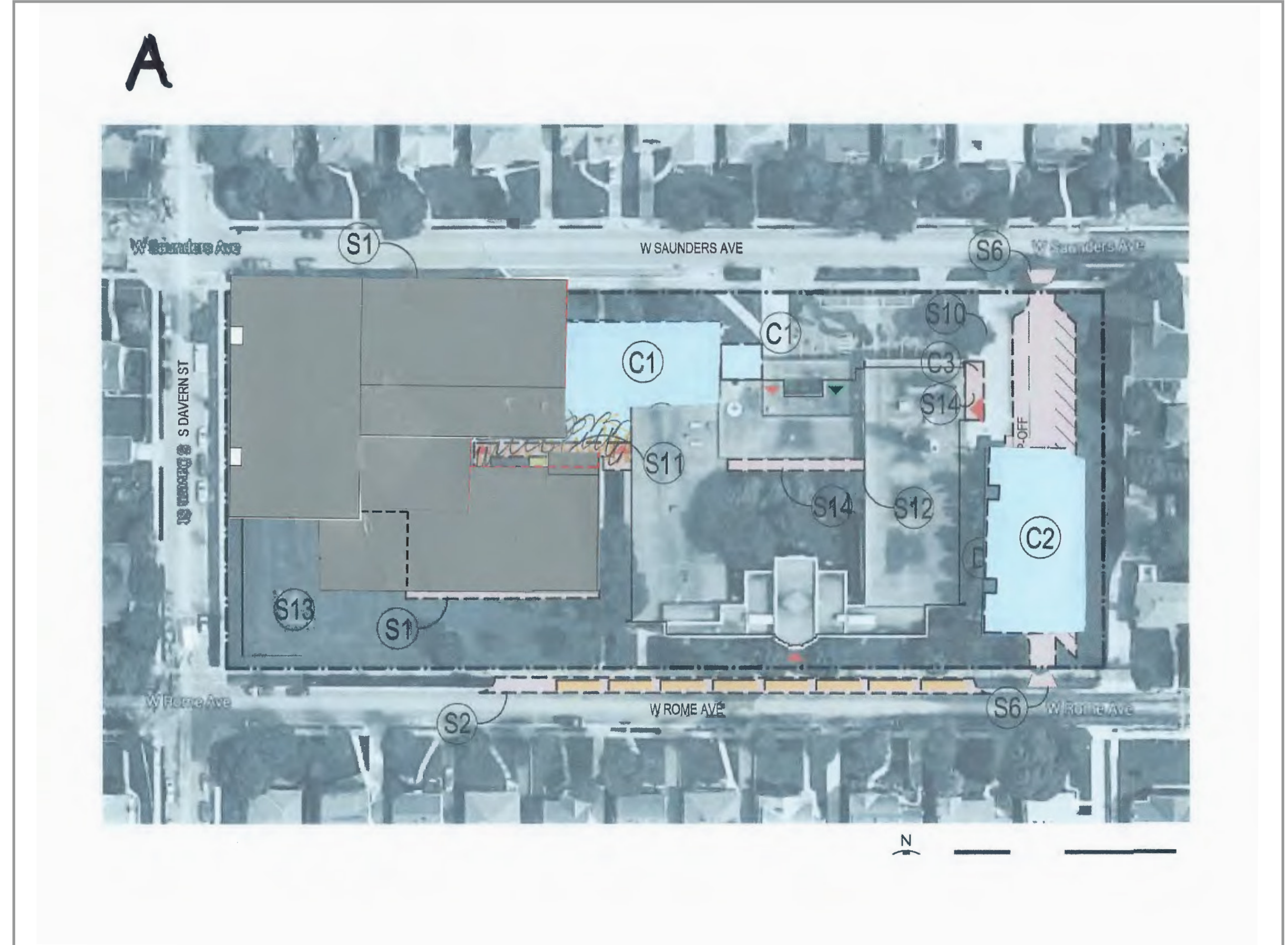
Sketch A: This is similar to the one we gave you – enlarging the existing gym and building two stories on the south east side of the school to provide for more classrooms. Some parking would remain on that side of the school. More parking could be added from cutouts along Saunders. Building a translucent roof over the corridor will add plenty of light and energy savings. This area is rarely used for recreation.
